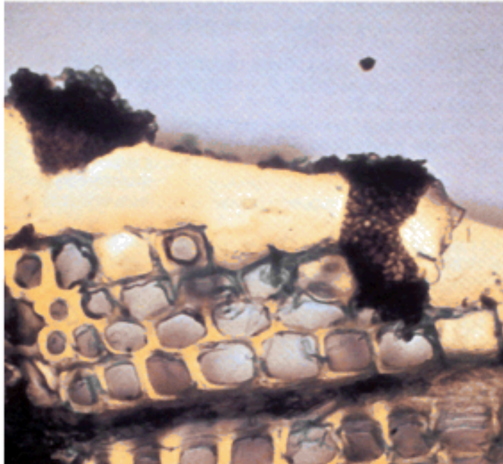
Figure 1.2: action of blue fungus that during its development succeeds in breaking through the film of coating and reach the surface.
